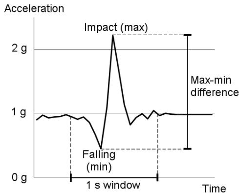
Figure 1: Acceleration pattern during a fall.
